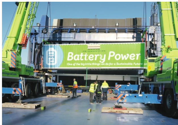
Above: Johan Stranne inside the battery unit. Right: The 1 MWh battery unit, equal to the power of about 12 Tesla cars and with a weight of 30 tonnes, is placed on the weather deck to fit.
